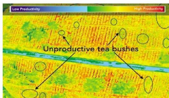
Figure 5- Tea plantation health mapping by Multi-spectral imaging ©TCS.
