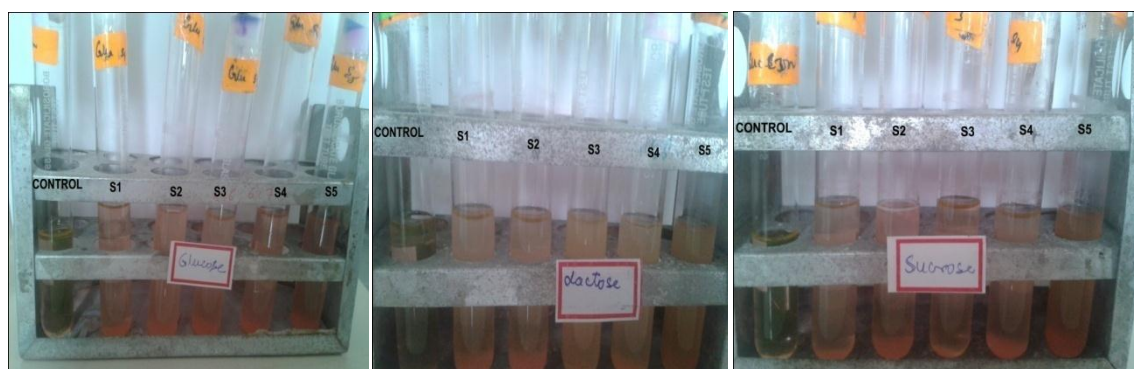
Effect of carbon source( Glucose, Lactose,Sucrose respectively) on decolorization of Eosin Yellow dye
