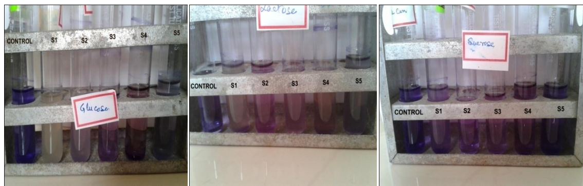
Effect of carbon source( Glucose, Lactose,Sucrose respectively) on decolorization of Crystal Violet dye
