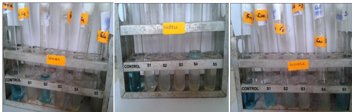
Effect of carbon source( Glucose, Lactose,Sucrose respectively) on decolorization of Methylene Blue dye
