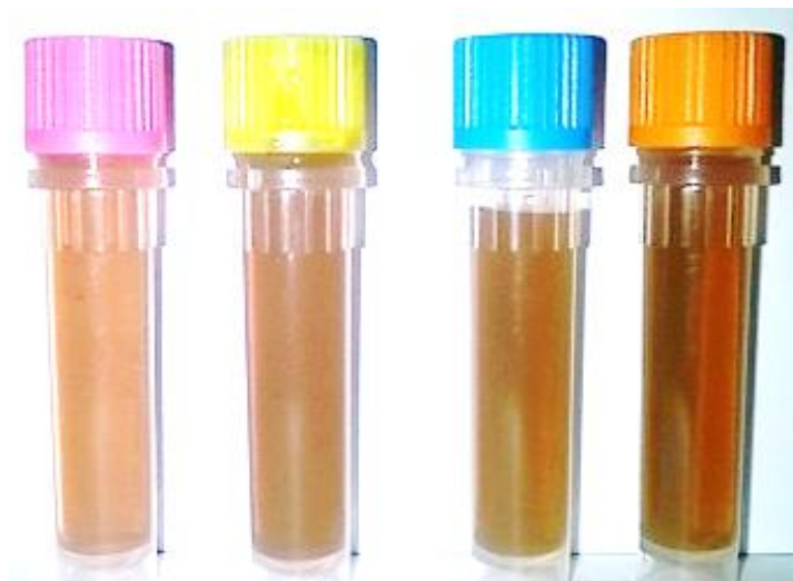
Figure 2: Synthesized silver nanoparticles exhibit a characteristic dark brown color.
